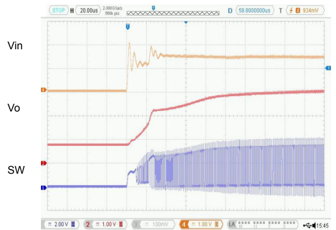
6. Start-up Waveform(VIN=2.4V, Rs=0.12Ω)
