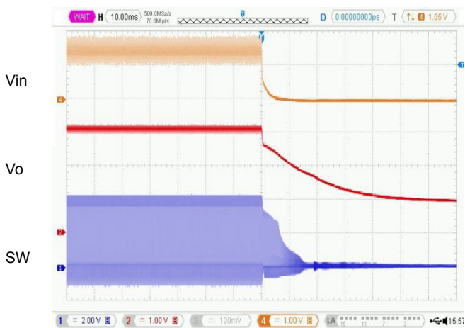
7. Shut-down Waveform(VIN=2.4V, Rs=0.12Ω)
